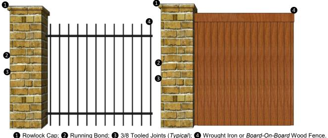
1 Rowlock Cap; 2 Running Bond; 3 3/8 Tooled Joints (Typical); 4 Wrought Iron or Board-On-Board Wood Fence.
