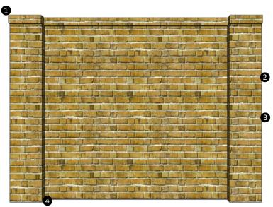
1 Rowlock Cap; 2 Running Bond; 3 3/8 Tooled Joints (*Typical*); 4 Concrete Footing/Mow Strip.
